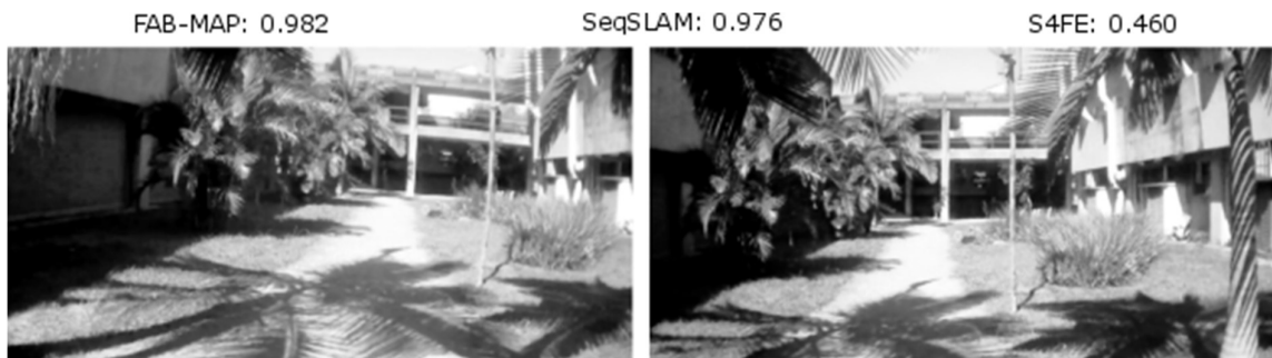
Figure 4.11 Sample of true positive returned by FAB-MAP, SeqSLAM and S4FE for the Parrot ArDrone 2.0 dataset with their coefficients p(L_i|Z^k) , \mu and \eta , respectively. Image generated by the author.
