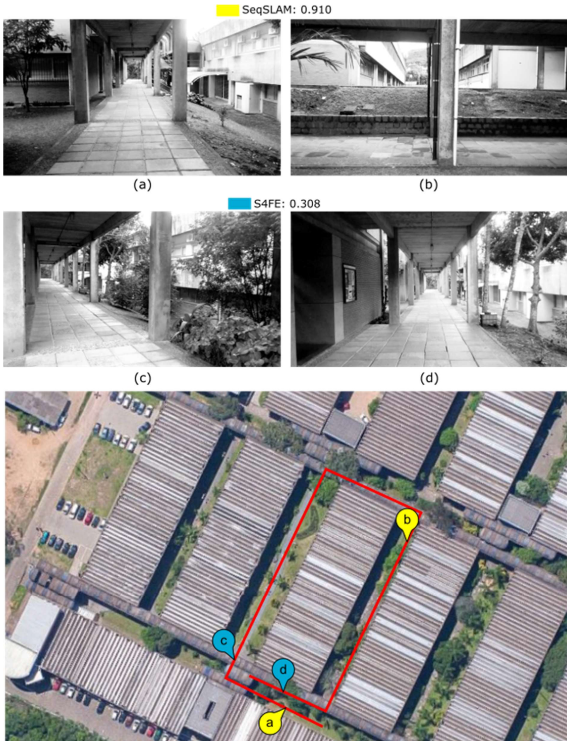
Figure 4.10 Samples of false positive obtained by SeqSLAM and S4FE in the handheld camera dataset with their coefficients \mu and \eta , respectively. FAB-MAP did not return any false positive. Image generated by the author.
